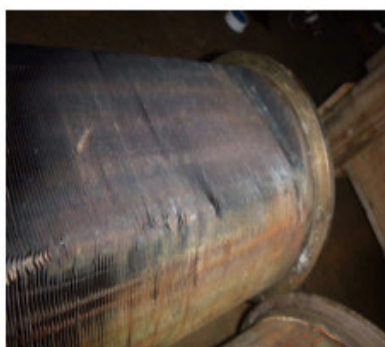
Carbon-choked fins before cleaning
