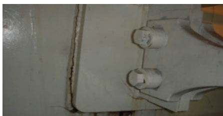
Top bracing detached from hull
