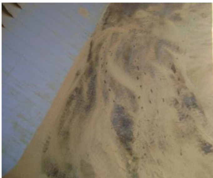
Damaged wheat cargo due to water ingress
