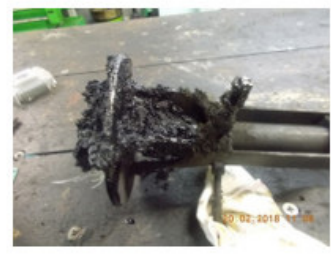
Observation 2: the burner nozzle and igniting rods were fully immersed in/ covered with carbon deposits.
